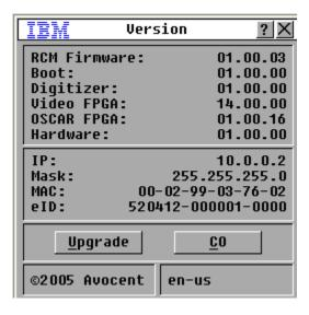
4. Click Upgrade. Type in the IP Address of the TFTP server where you have stored the firmware file. Type in the filename.
