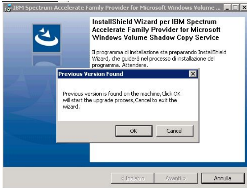
Figure 6. IBM Spectrum Accelerate Family VSS Provider Installation Wizard Welcome panel with upgrade confirmation
