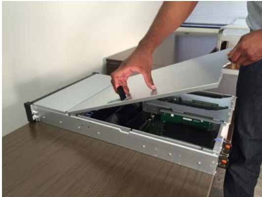
Figure 25. Replacing the SV1 cover
