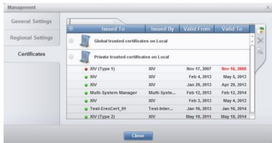
Figure 2. Importing certificates into the local truststore
