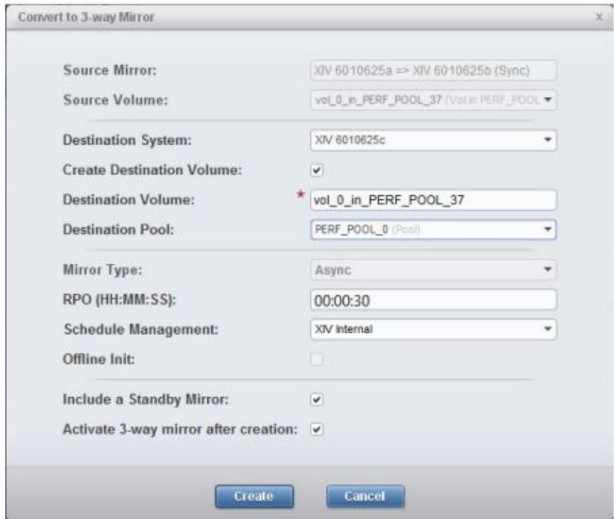
Figure 43. Convert to 3-way Mirror definition window
