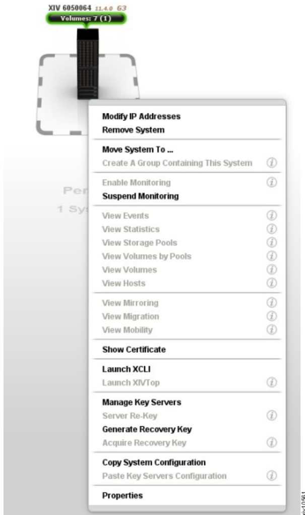
Figure 30. Right-click the XIV system and select Generate Recovery Key from the menu.
