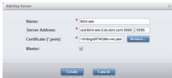
Figure 22. Adding a key server
