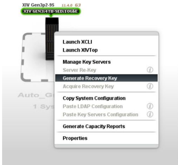
Figure 25. Right-click the XIV system and select Generate Recovery Key from the menu.
