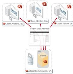
• A separate server that consolidates multiple content nodes — local, remote, or cloud-based file systems — into a single view and enables management of user access and file transfers across all nodes.
