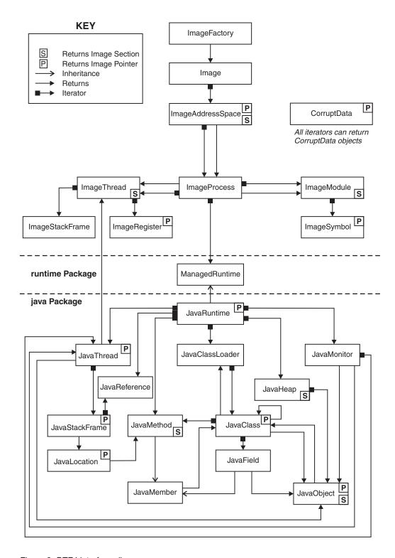
Figure 3. DTFJ interface diagram
